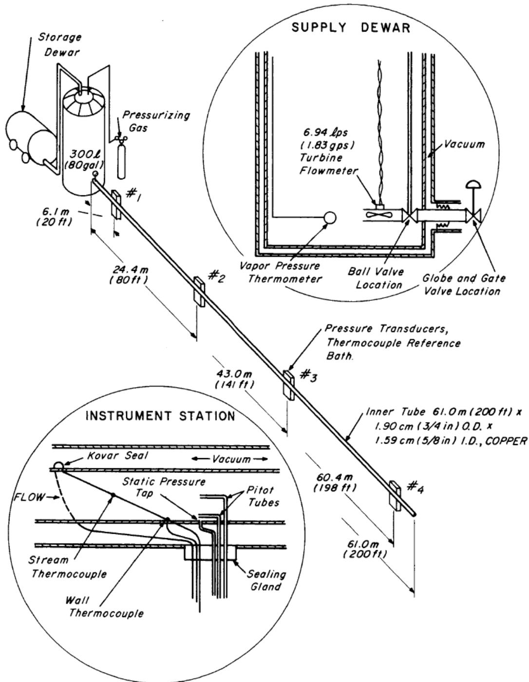
The fluid within the supply dewar was either (1) pressurized and allowed to come to approximate thermal equilibrium at that pressure (“saturated”), or was (2) quickly pressurized from saturation at atmospheric pressure (“subcooled”).
