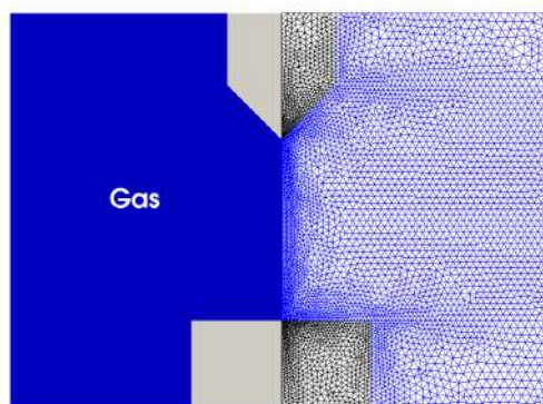
Figure 1: Domain and mesh for the pin to plane arc simulation. The mesh consists of 9,664 cells. The anode (top electrode) is conical in shape with base diameter of 0.6 mm, and the cathode (bottom electrode) is cylindrical (diameter 1 mm).
